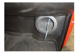
After securing all the allen bolts and the 7/16 nuts run your speaker wire into the speaker pod
