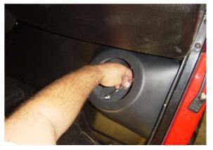
Once the holes are drilled, mount the kickpanel using the supplied hardware
