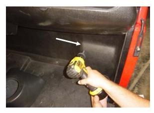
After marking the holes, drill them using a 1/4" drill bit
