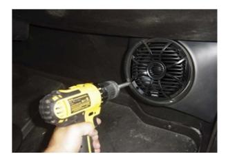
After attaching the speaker wires to the speaker, install the speaker into the Wet Sounds pod.
